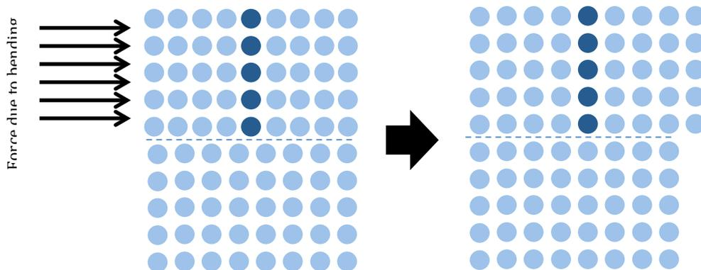
Motion of dislocation with increased force. Plans of atoms slide over one another to reach the edge
