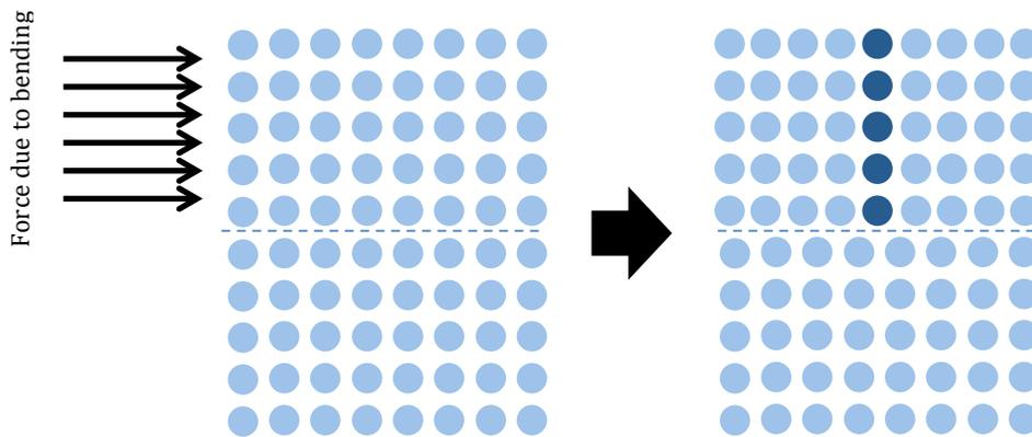
Image of dislocation creation in a metal. Dark blue atoms show the planar defect created.
